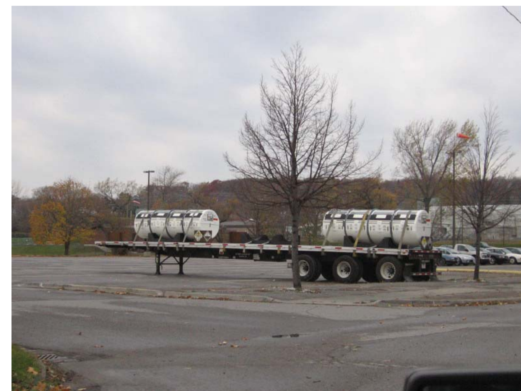
Two UF 6 drums left on a trailer in a publicly accessible parking lot
