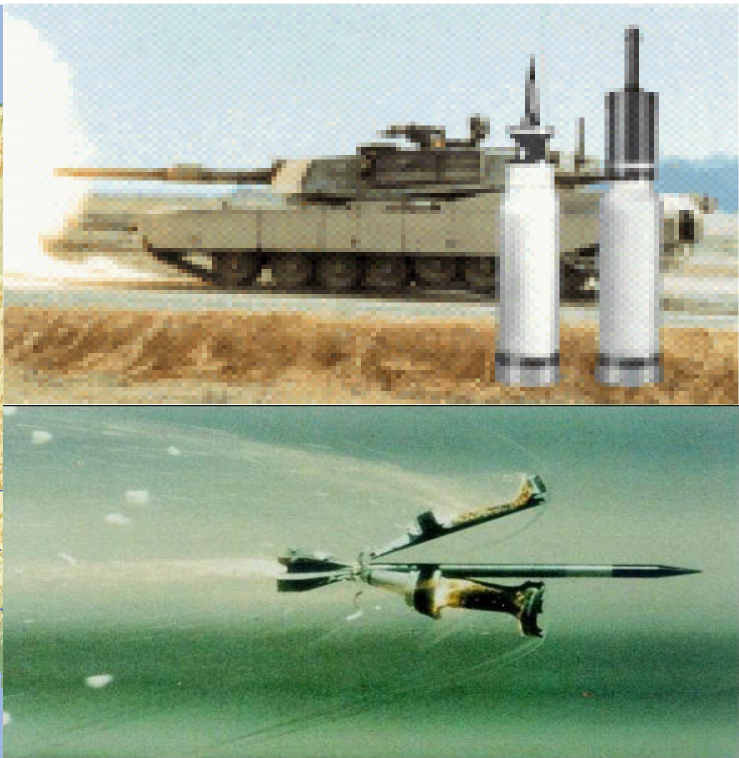
120mm DU Anti-tank Long Rod Penetrator
