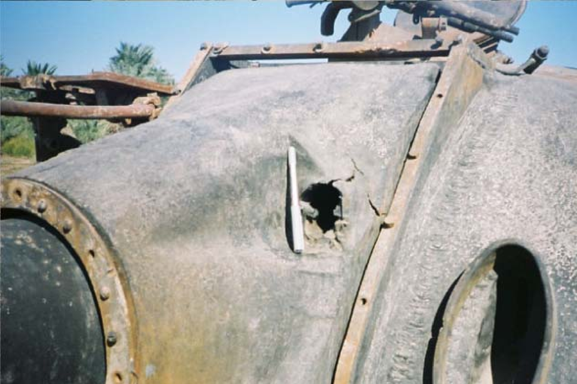
Uranium penetrator passes through 4+ inches of steel
