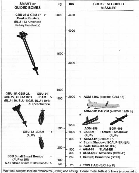
Warhead weights include explosives (~20%) and casing. Dense metal ballast or liners (suspected to be DU) estimated to be 50-75% of warhead weight - necessary to double the density of previous versions. AUP = Advanced penetrators. S/CH = Shaped Charge. BR = BROACH Multiple Warhead System (S/CH+AUP). P = older 'heavy metal' penetrators. © Dai Williams 2002
